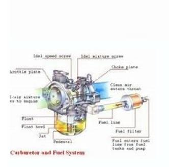
Motorcycle carburetor parts and function pdf. Motorcycle carburetor parts and their functions. Motorcycle carburetor parts and functions.
